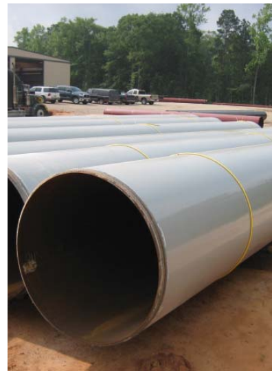
Pipe coated with 30 mils of Protal 7900HT.
